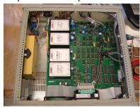
Signal processor and display unit - redesign and manufacture of circuit boards
